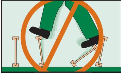
Never stack building materials over unsheathed I-joists. Stack only over beams or walls.
